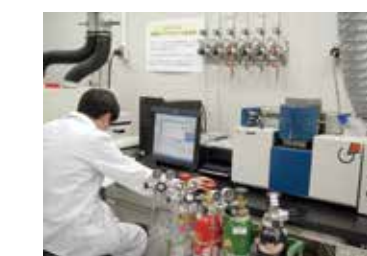
Examining inclusion of high fructose corn syrup in foods by using IRMS
