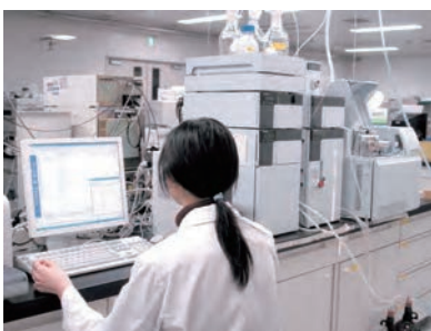
Analysis of feed for mycotoxins using liquid chromatography mass spectrometer (LC-MS)
