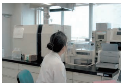
Analysis of fertilizer for lead and cadmium using ICP-MS
