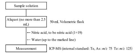
Figure 3 Flow sheet for arsenic in fertilizers (Measurement procedure)
