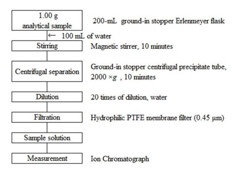
Figure Flow sheet for chlorine in fertilizers
