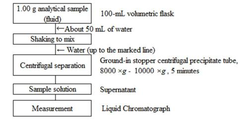
Figure 2 Flow sheet for urea nitrogen in fertilizers
