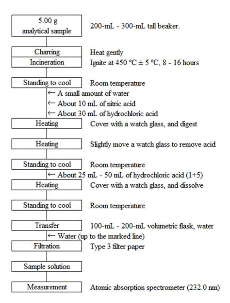
Figure Flow sheet for nickel in fertilizers
