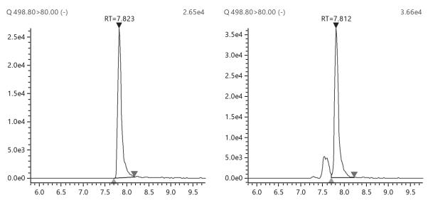
Standard solution (20 ng/mL as PFOS) Sample solution (composted sludge fertilizer)
