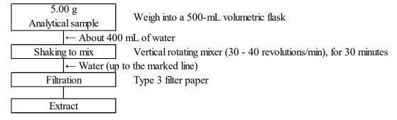
Figure 1-1 Flow sheet for urea nitrogen (Extraction procedure (4.1.1))
