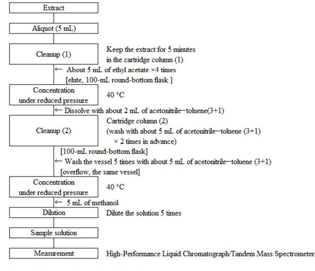
Figure 2 Flow sheet for residue agrichemicals multicomponent analysis
