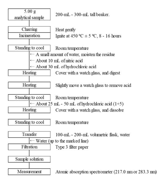
Figure Flow sheet for lead in fertilizers
