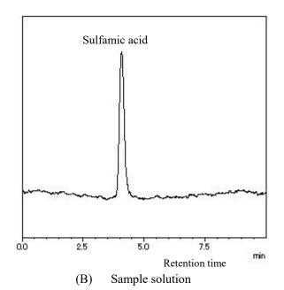
(The equivalent of 0.1 % of mass fraction as sulfamic acid is added to a compound fertilizer)
