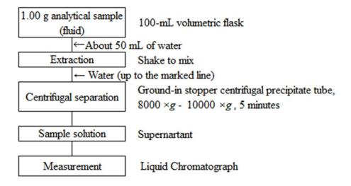
Figure 2 Flow sheet for biuret nitrogen in fertilizers
