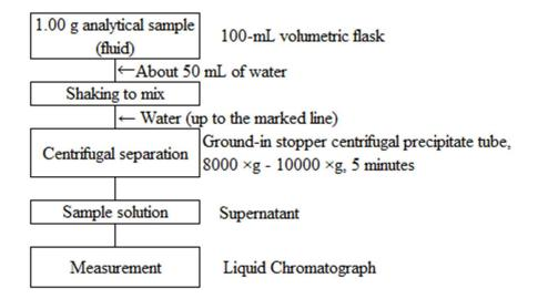
Figure 2 Flow sheet for dicyandiamide nitrogen in fertilizers (Extraction procedure (4.1.2) and measurement)
