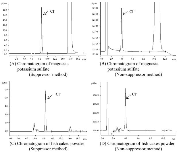
Reference diagram: IC chromatogram of chloride ion (Peak: 1.chloride ion (Cl<sup>-</sup>))
