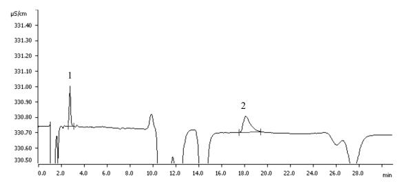
(A) Mixture standard solution (the equivalents of 60 ng (3 mg/L, 20 μL) as sulfamic acid and ammonium thiocyanate, respectively)
