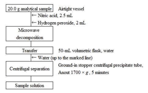
Figure 1 Flow sheet for chromium in fluid sludge fertilizers (Extraction procedure)
