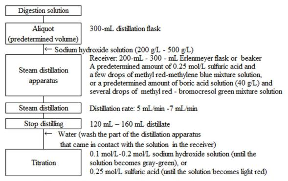
Figure 3 Flow sheet of the testing method for heat buffer solution soluble nitrogen in methylolurea polymerization fertilizers (Distillation and measurement procedure)
