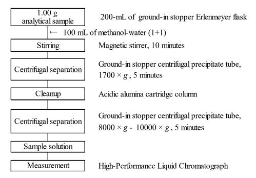
Figure Flow sheet for 2-amino-4-chloro-6-methylprimidine (AM) in fertilizers.
