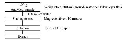
Figure 1-2 Flow sheet for urea nitrogen (Extraction procedure (4.1.2))
