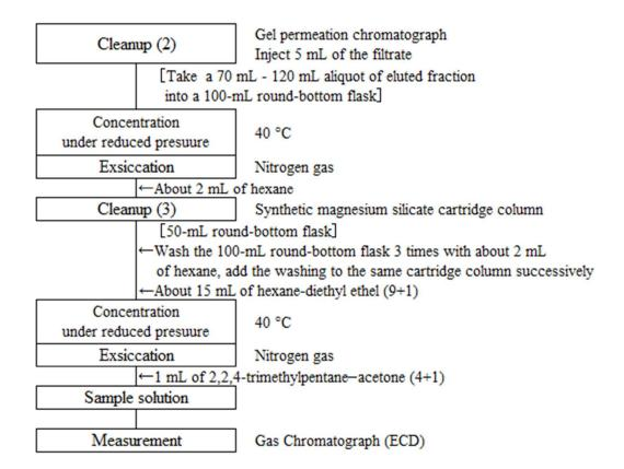
Figure 3 Flow sheet for residue agrichemicals multicomponent analysis
