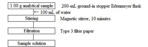
Figure 1 Flow sheet for chroline in potassium sulfate, etc. (Extraction procedure)
