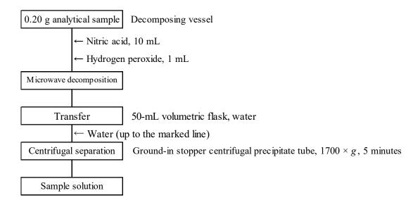
Figure 2 Flow sheet for lead in fertilizers except fluid sludge fertilizers (Extraction procedure)
