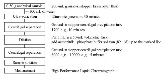
Figure Flow sheet for melamine in fertilizers containing organic matter
