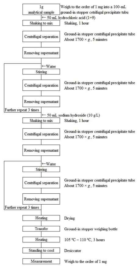
Figure 2 Flow sheet of the testing method for humic acid in humic acid salt fertilizers
