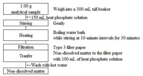
Figure 1 Flow sheet of the testing method for heat buffer solution soluble nitrogen in methylolurea polymerization fertilizers (Extraction procedure)
