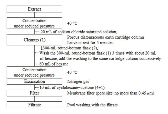
Figure 2 Flow sheet for residue agrichemicals multicomponent analysis
