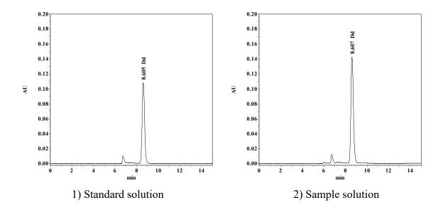
Reference diagram HPLC chromatogram of dicyandiamide (Dd)
