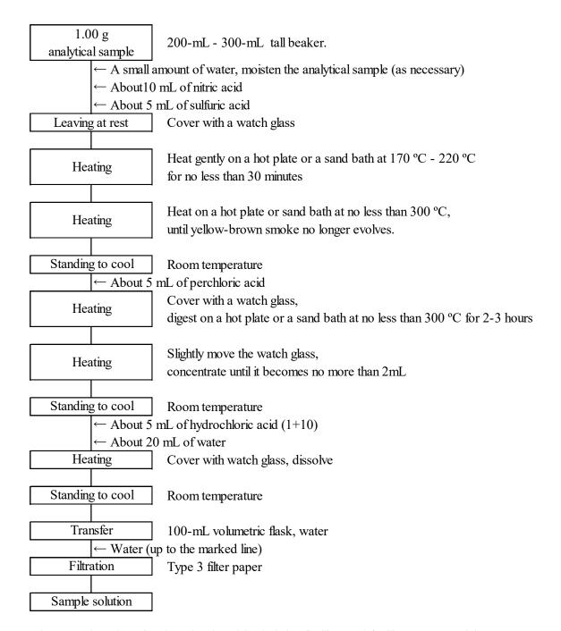
Figure 1 Flow sheet for chromium in calcined sludge fertilizer and fertilizers not containing organic matters (Extraction procedure)
