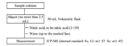
Figure 3 Flow sheet for chromium in fertilizers containing organic matters (Measurement procedure)
