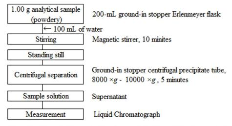
Figure 1 Flow sheet for guanidine nitrogen in fertilizers (Extraction procedure (4.1.1) and measurement)
