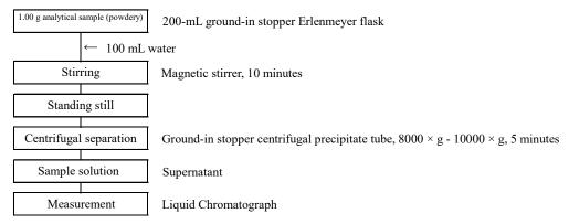
Figure Flow sheet for 3,4-dimethylpyrazole phosphate (DMPP) in fertilizers (Extraction procedure (4.1.1) and measurement)
