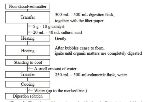
Figure 2 Flow sheet of the testing method for heat buffer solution soluble nitrogen in methylolurea polymerization fertilizers (Kjeldahl digestion procedure)
