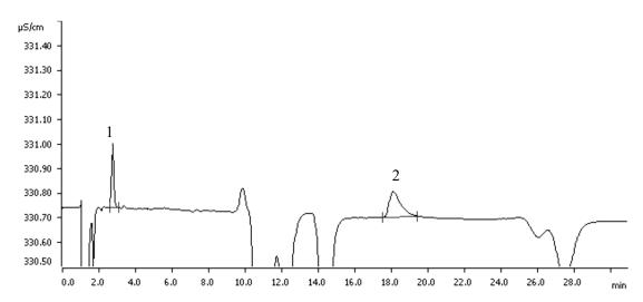
(A) Mixture standard solution (the equivalents of 60 ng (3 mg/L, 20  $\mu$ L) as sulfamic acid and ammonium thiocyanate, respectively)
