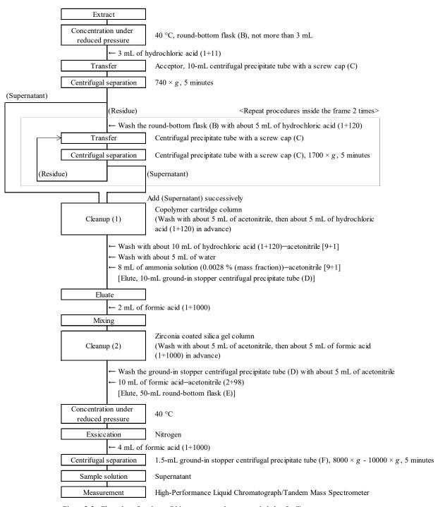
Figure 2-2 Flow sheet for clopyralid in compost and composted sludge fertilizers (Cleanup (1), cleanup (2) and measurement procedures)
