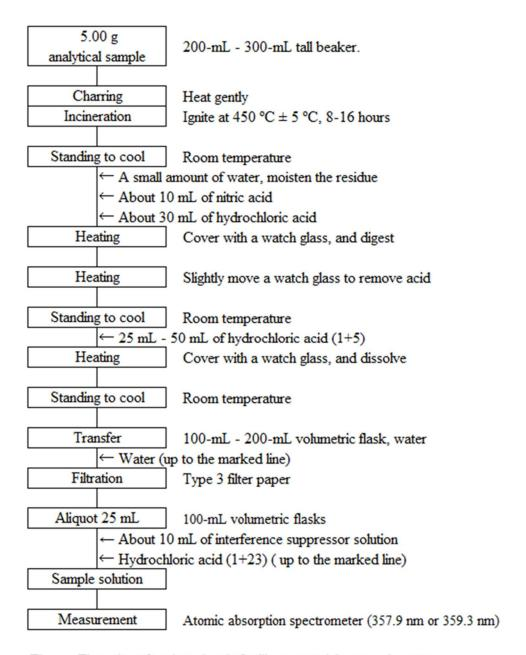
Figure Flow sheet for chromium in fertilizers containing organic matters
