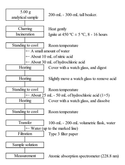
Figure Flow sheet for nickel in fertilizers
