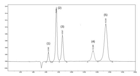
Reference diagram: HPLC chromatogram of the mixture standard solutions for the calibration curve preparation (10 mg/L for each)
