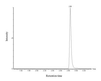
Reference diagram: SRM chromatograms of clopyralid Clopyralid standard solution (the equivalents of 50 pg as clopyralid)
