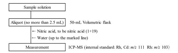
Figure 3 Flow sheet for cadmium in fertilizers (Measurement procedure)
