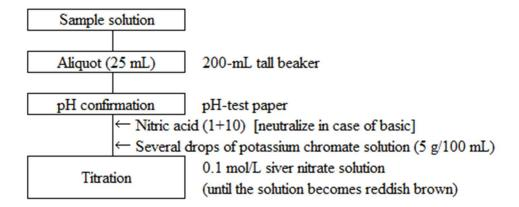
Figure 2 Flow sheet for chroline in potassium sulfate, etc. (Measurement procedure)
