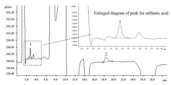
(B) Sample solution (the equivalents of 0.25 % (mass fraction) (2500  $\mu$ g/g) as sulfamic acid and ammonium thiocyanate added in ammonium sulfate, respectively)
