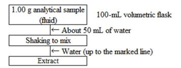
Figure 1-2 Flow sheet for sulfamic acid in fertilizers (Extraxction procedure (4.1.2))
