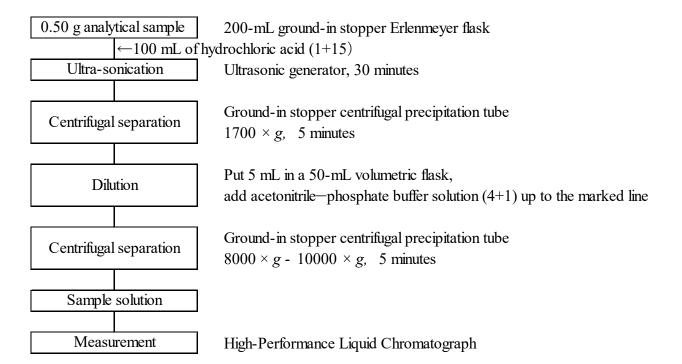
Figure Flow sheet for melamine derivations in fertilizers
