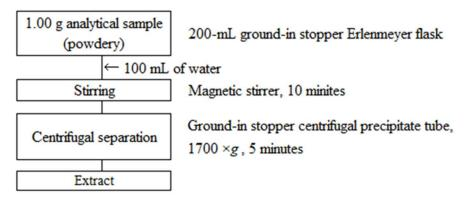
Figure 1-1 Flow sheet for ammonium thiocyanate in fertilizers (Extraction procedure (4.1.1))
