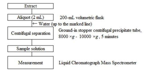
Figure 2 Flow sheet for sulfamic acid in fertilizers
