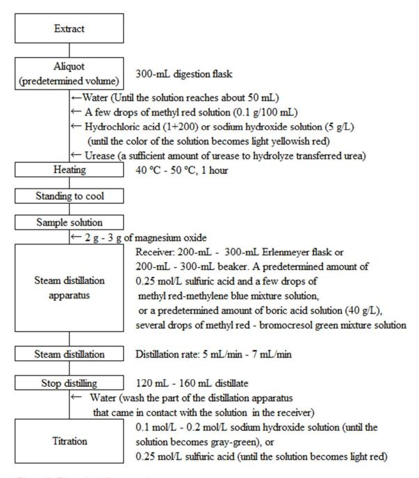
Figure 2 Flow sheet for urea nitrogen
