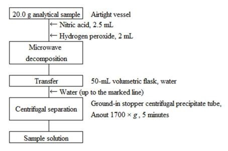
Figure 1 Flow sheet for cadmium in fluid sludge fertilizers (Extraction procedure)
