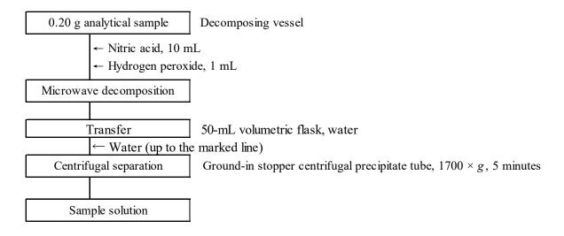
Figure 2 Flow sheet for cadmium in fertilizers except fluid sludge fertilizers (Extraction procedure)
