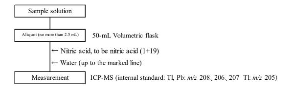
Figure 3 Flow sheet for lead in fertilizers (Measurement procedure)
