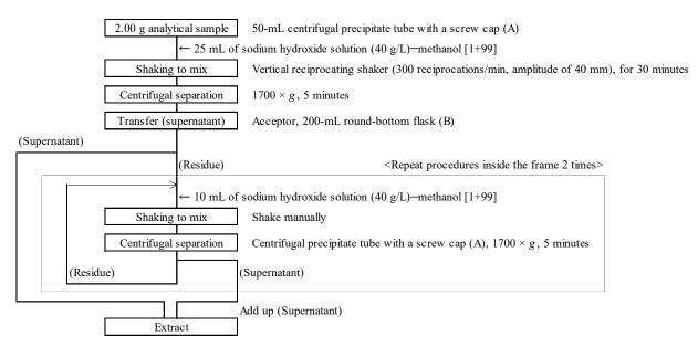
Figure 2-1 Flow sheet for clopyralid in compost and composted sludge fertilizers (Extraction procedure)
