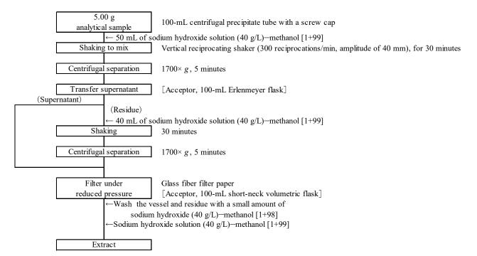
Figure 1 Flow sheet for clopyralid in compost and composted sludge fertilizers (Extraction procedure)
