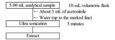
Figure 1 Flow sheet for residue agrichemicals multicomponent analysis ((1): simultaneous analysis of 6 kinds of agrichemicals) in fertilizers (Extraction procedure)
