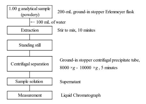
Figure 1 Flow sheet for guanylurea nitrogen in fertilizers (Extraction procedure (4.1.1) and mesurement)
