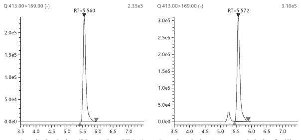
Standard solution (20 ng/mL as PFOA) Sample solution (composted sludge fertilizer) Reference diagram 2: MRM chromatograms of PFOA
