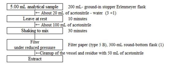
Figure 1 Flow sheet for residue agrichemicals multicomponent analysis
