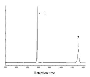
(A) Mixture standard solution (The equivalents of 100 ng (10  $\mu$ g/mL, 10  $\mu$ L) as nitrous acid and ammonium thiocyanate, respectively)
