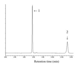
(A) Mixture standard solution (The equivalents of 100 ng (10  $\mu$ g/mL, 10  $\mu$ L) as nitrous acid and ammonium thiocyanate, respectively)
