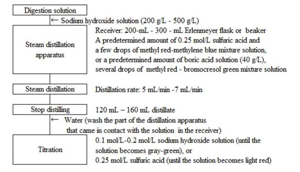
Figure 3 Flow sheet for cold buffer solution soluble nitrogen testing method in formaldehyde processed urea fertilizers
