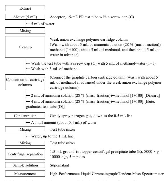
Figure 2-2 Flow sheet for organofluorine compounds in sludge fertilizers (Cleanup and measurement procedures)
