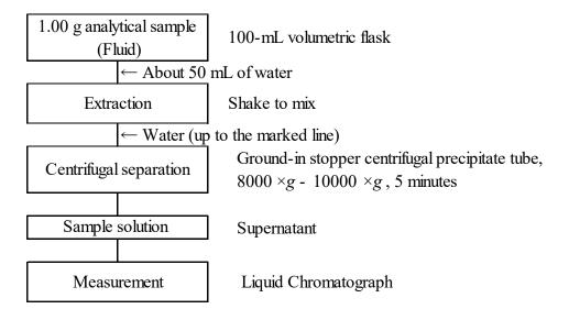
Figure 2 Flow sheet for guanylurea nitrogen in fertilizers (Extraction procedure (4.1.2) and mesurement)
