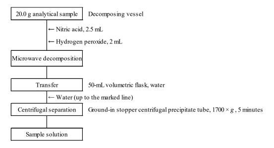
Figure 1 Flow sheet for arsenic in fluid sludge fertilizers (Extraction procedure)
