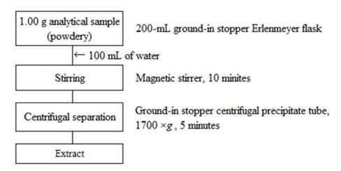
Figure 1-1 Flow sheet for sulfamic acid in fertilizers (Extraxction procedure (4.1.1))
