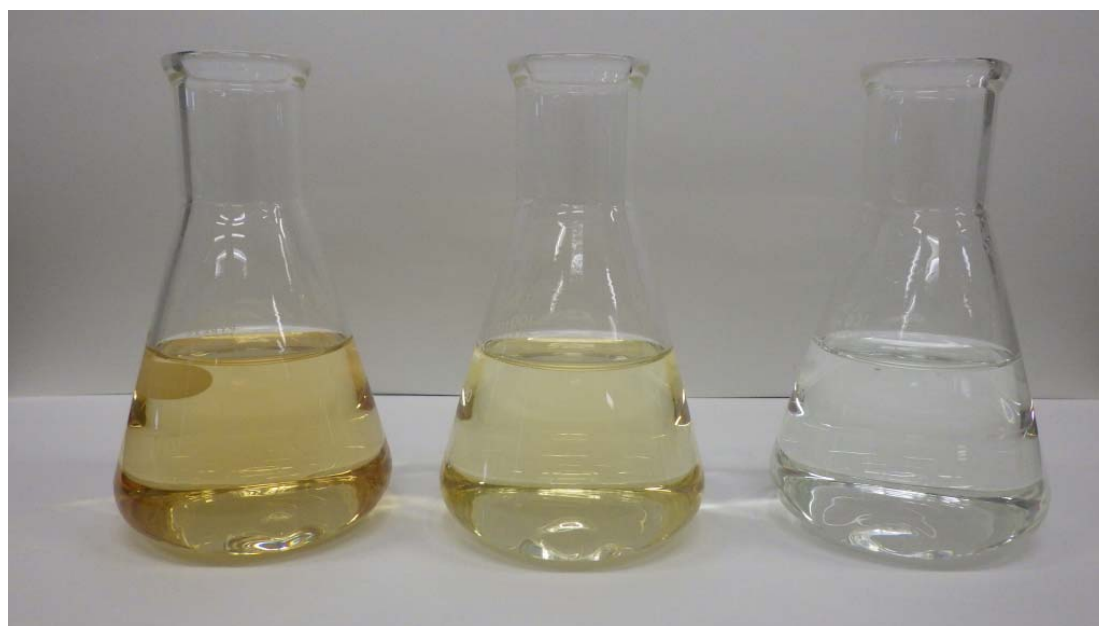
Fig.2 Citrate solution extract of chemical fertilizer
