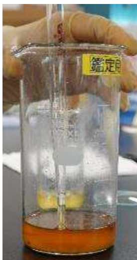
5. Transfer all floating solids in the beaker to another beaker using komagome pipette etc.
