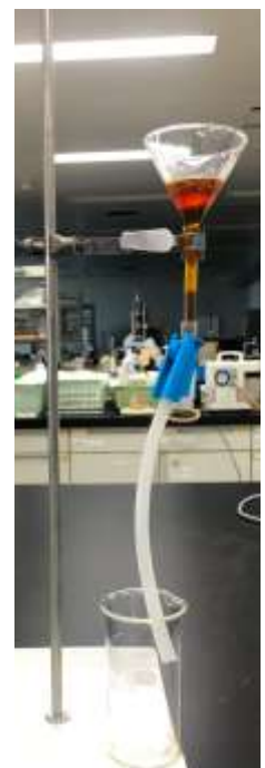
Fig.1 Density separation using funnel
