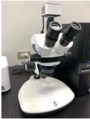
3. visual assess and observation by stereoscopic microscope
