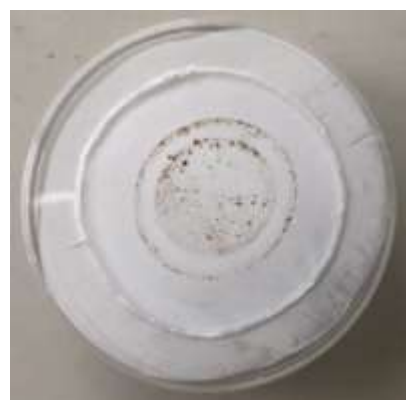
2-2. Set a membrane filter to folder and desiccate it
