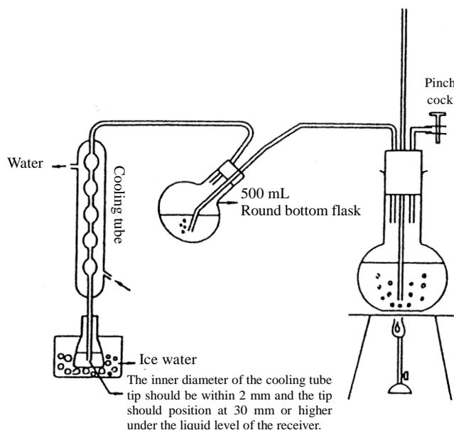
Figure 12.1.1-3 Distillation apparatus
