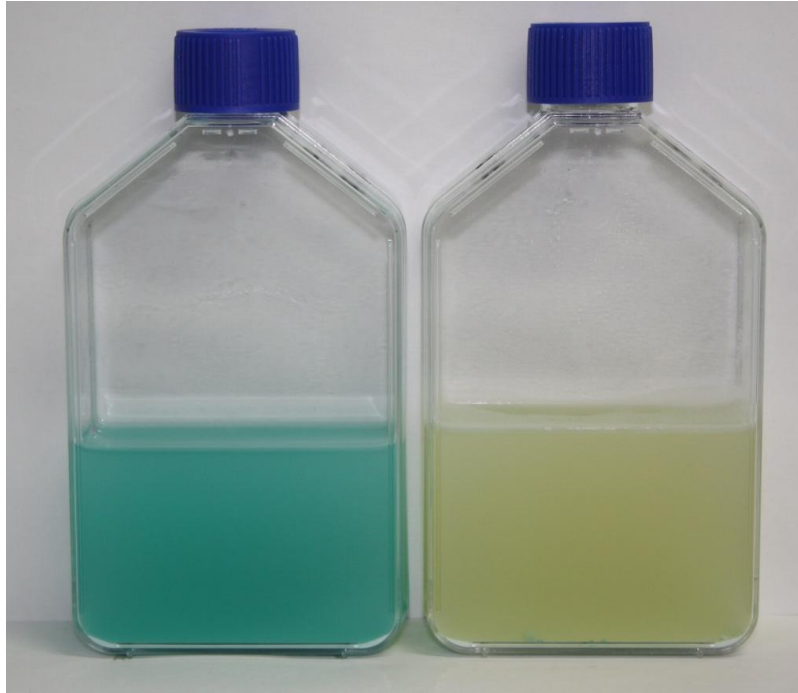
Figure 18.1-7 Example of selective enrichment culture (1: Hajna tetrathionate broth) (Left: before use Right: after cultivation)
