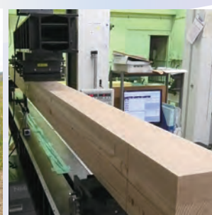
Measurement of flexural strength of structural laminated timber
