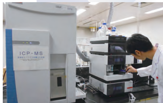
Analysis of lead and cadmium in fertilizer by using ICP-MS
