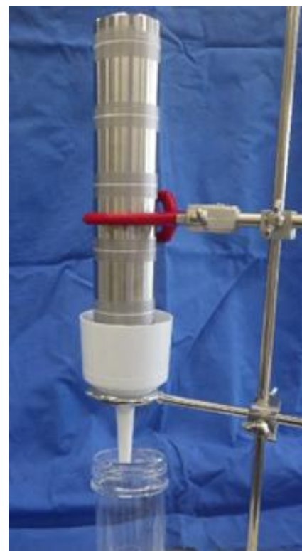
Figure 2 Image of a soil column
